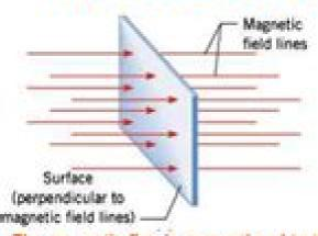
The magnetic flux is proportional to the number of field lines that passthrough a surface.
