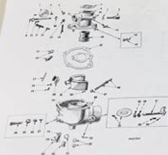
Fig. 2. Exploded view of International Model E-12, 1.54" updraft and E-13, 1.28" updraft Carburetors.
