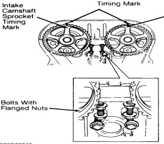
Exhaust Camshaft Sprocket Timing Mark
