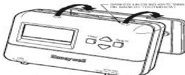
A ENGAGE TABS AT TOP OF THERMOSTAT WITH SLOTS ON WALLPLATE.
