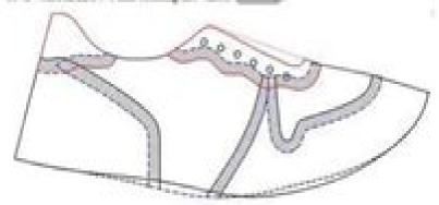
The combined model, in which the vamp and facing parts are leather, and the quarter are tentile (Model 3).
