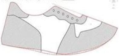
The shor model made of leather, in which case the shor upper comists of separate parts, seven with standard 7-8 mm stacking allowances (Model 2).
