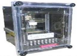
VAPM31 Relay is used for detection of failure or inadvertent removal of voltage transformer secondary fuses and for prevention of incorrect tripping of circuit breakers.
