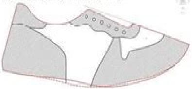
The shor model made of leather, in which case the shor upper comists of separate parts, seven with standard 7-8 mm stacking allowances (Medel 2).
