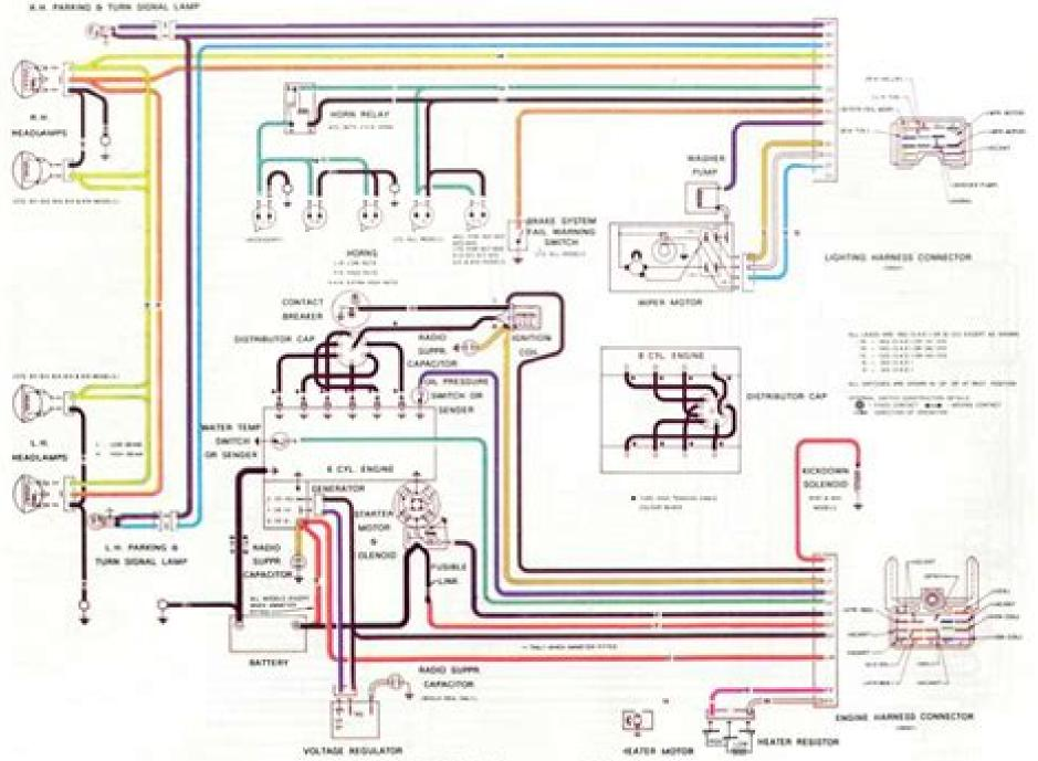
Fig. 1. Engine Compartment Wiring
