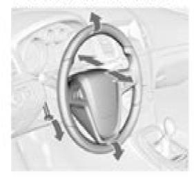
Unlock lever, adjust steering wheel, then engage lever and ensure it is fully locked.
