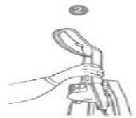
Line up the handle to the upper body of the machine and slide into place.
