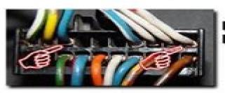
B5 = VTEC Pressure Switch B19 = Knock Sensor
