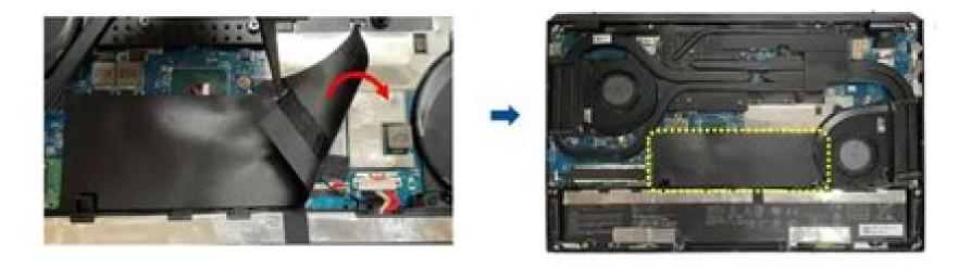
Install the base cover at a slight tilt at upper side first, and then press
