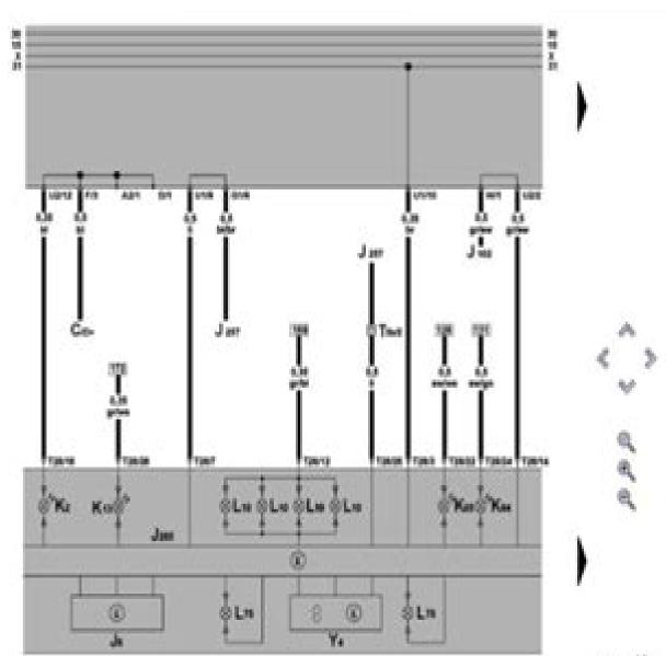
Dash panel insert, warning lamp, odometer display
