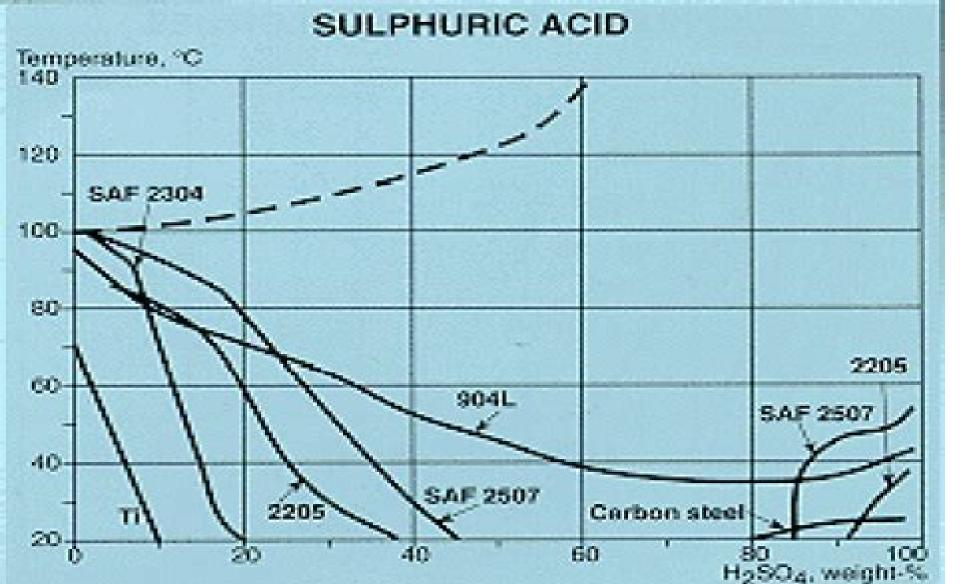
Isocorrosion diagram, 0.1 mm/year, for duplex stainless steels, titanium and carbon steel in naturally aerated sulphuric acid of chemical purity. Broken-line curve represents the boiling point.
