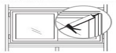
STEP 3. Fill the gags, interior, exterior and around the perimeter of the window between the mainframe and wall with an approved polyurathene based scalant such as Vulkem® or 100% silicone window and door caulic.
