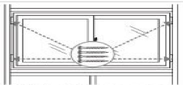
STEP 2. Secure window using 2-1/4" screws fastened through the pre-punched installation holes located on the side walls las shown above.
