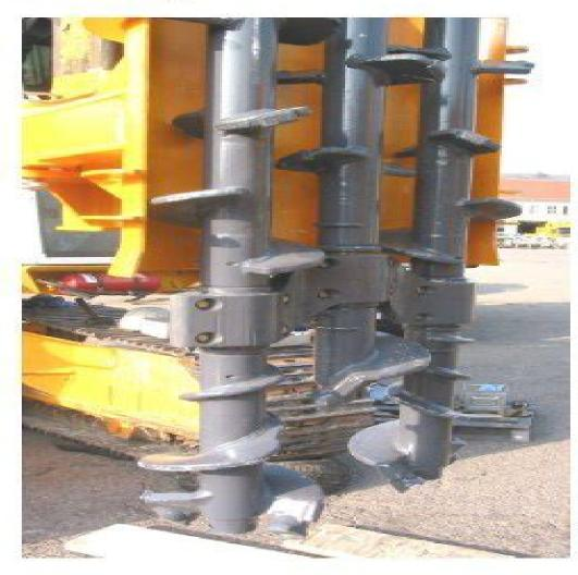
Mixing self-hardening sturry in-situ with native soil (SMW) is a cost-effective technique for the construction of walls for groundwater control (cut-off walls), walls for excavation support (retaining walls) as well as for ground improvement.
