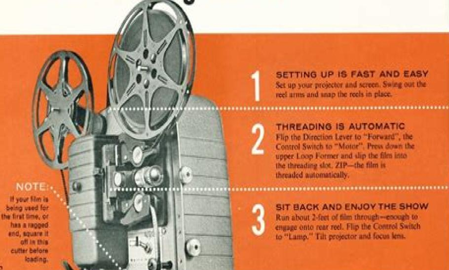
SETTING UP IS FAST AND EASY Set up your projector and screen. Swing out the reel arms and map the reels in place.
