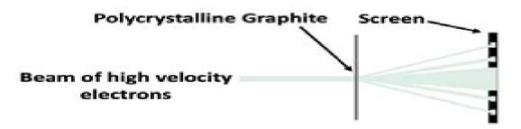
A circular pattern of rings is observed. The wavelength of electrons must be approximately equal to the spacing between the atoms in the polycrystalline graphite. This is true and the value is around 10<sup>-10</sup> m.
