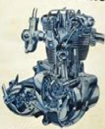
UNIT CONSTRUCTION 650 C.C. TWINS 1730 and TRA - FROM ENGINE No. DO. 85000
