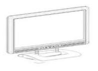
LCD monitor can be lay back 0" ~2" (positive and negative 2").
