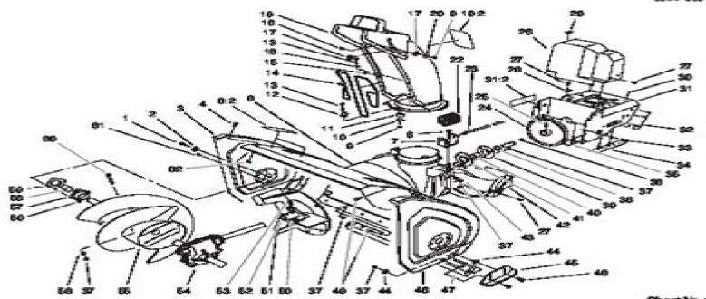
Housing and Engine Frame Assembly
