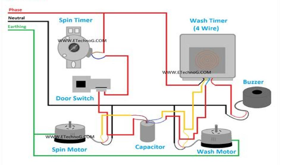
Washing Machine Wiring and Connection Diagram
