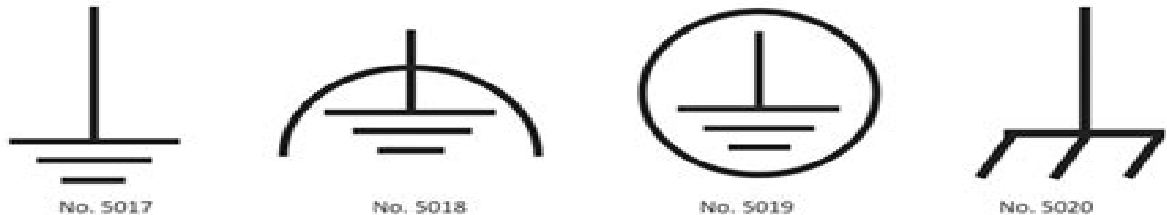
Figure 1: IEC 60417 ground symbols
