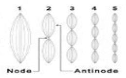
The wavelength of a standing wave can be found by measuring the length of two of the "bumps" on the string. The first harmonic only contains one bump, so the wavelength is twice the length of the individual bump.
