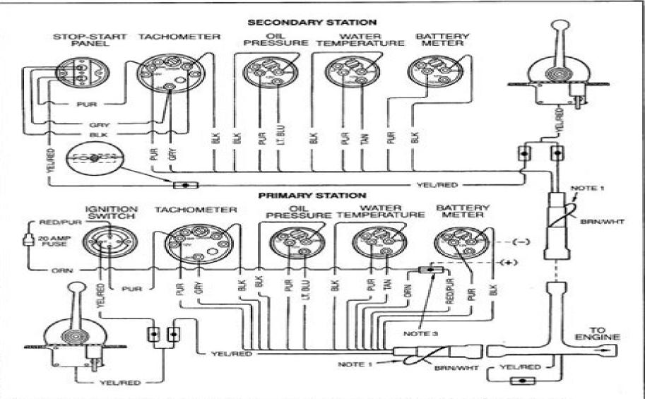
NOTE 1: Brown/white wire is taped back at instrument end. If installing on boat that is equipped with MerCruiser Stern Drive, brown/ white wire is connected to trim sender terminal block. If installing on Mercruiser Inboard, brown/white wire is taped back at engine end, or it may be used for an accessory (limit 5 amps).
