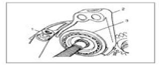
Unfasten caulking of countershaft nut, install input shaft 5th gear (1) and special tool to stop rotation of shafts, and then remove countershaft nut (2).
