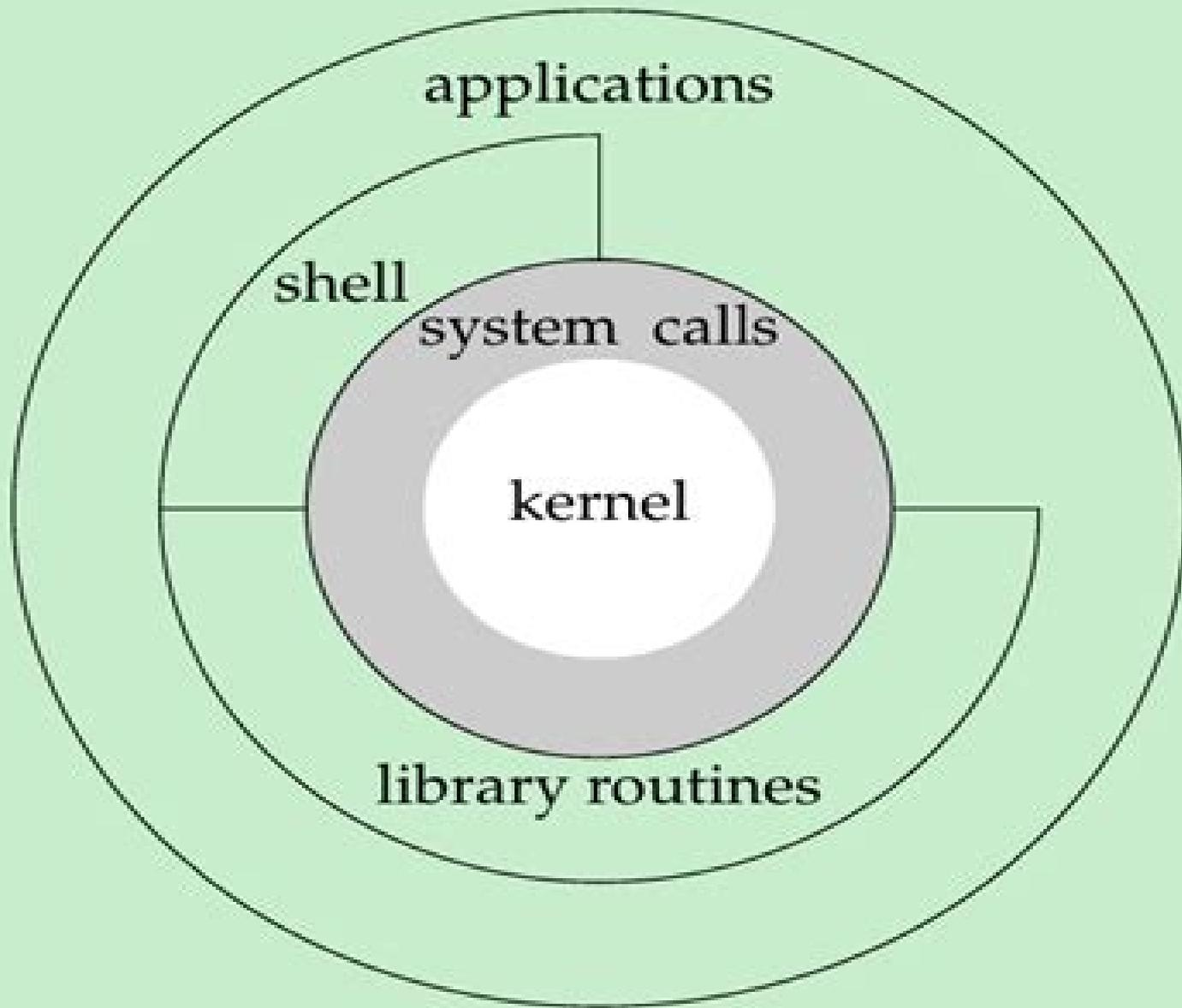
**Figure 1.1** Architecture of the UNIX operating system
