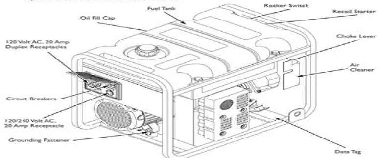
I 20 Volt AC, 20 Amp, Duplex Receptacles — May be used to supply electrical power for the operation of I 20 Volt AC, 20 Amp, single phase, 60 Hz electrical, lighting, appliance, tool and motor loads.
