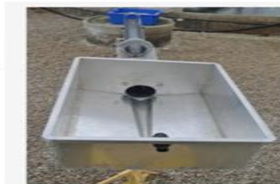
Figure 7 —Low-cost humane slaughter device for small to medium size aquaculture producers.
