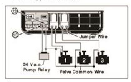
A CAUTION: To prevent pump damage due to "dead heading," connect a jumper wire from any unused zone terminal to a zone terminal with a valve connected.
