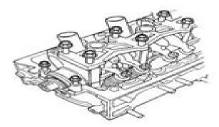
Tighten each boit two turns at a time, in the sequence shown below, to ensure that the rockers do not bind the valves.
