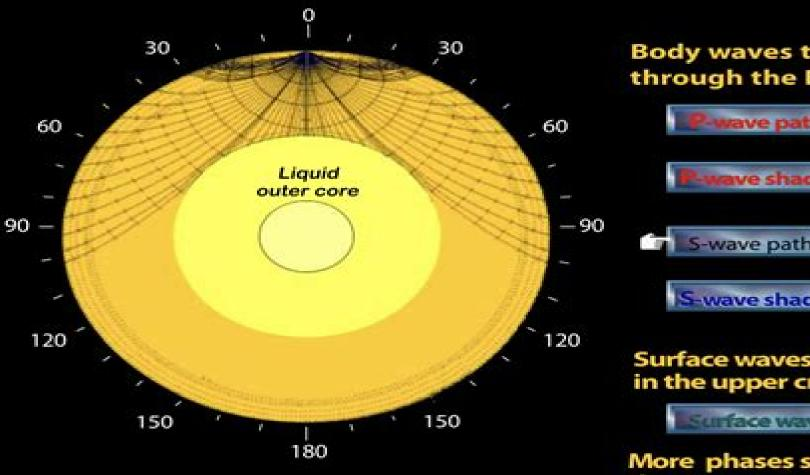
S-waves travel forward with a side-to-side shearing motion. Shearing waves cannot travel in a liquid, thus are unable to pass into the Earth's core. The paths through the mantle are curved due to wave refraction as the material properties change.
